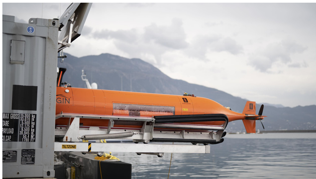
Figure 1. Autonomous Underwater Vehicle HUGIN during shore recovery: the underwater component of the mapping devices set used in Round 2 of Shell Ocean Discovery XPRIZE (Photography by XPRIZE).
