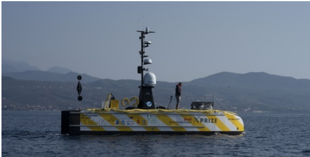
Figure 2. USV SEA-KIT ‘Maxlimer’ during the preparation to the final survey, Kalamata, Greece: the surface part of the mapping devices set used in Round 2 of Shell Ocean Discovery XPRIZE (Photography by XPRIZE).
